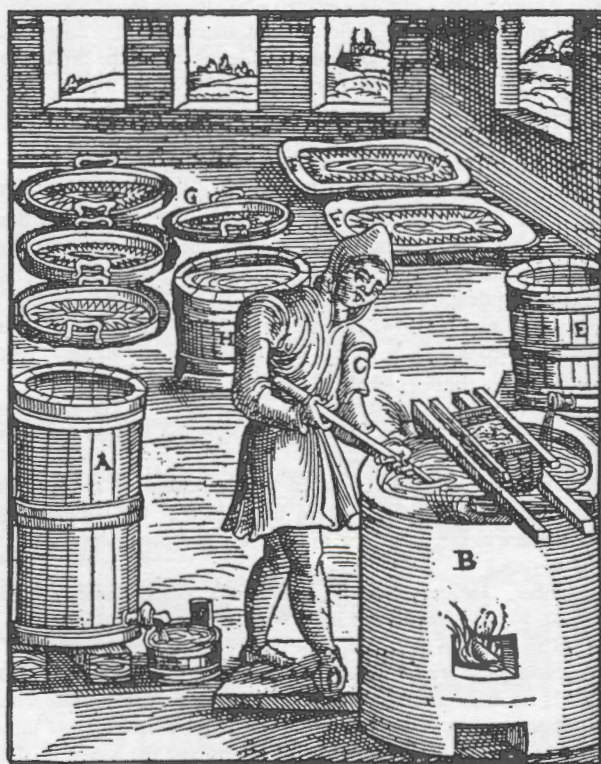
[130] [FIGURE 40.—PANS AND TUBS FOR CRYSTALLIZING SALTPETER]
